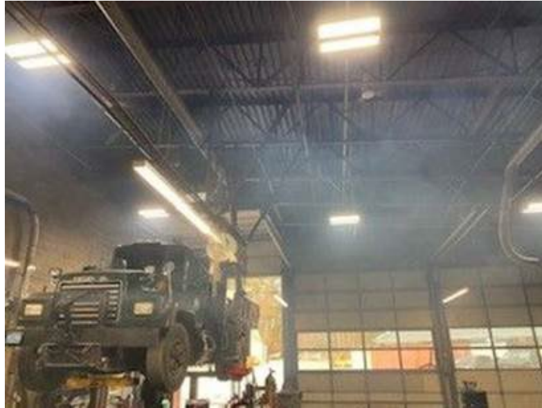
Photo: smoke in mechanics garage from repairs of truck. The garage door was open during repair and this demonstrates the poor ventilation and air quality.
